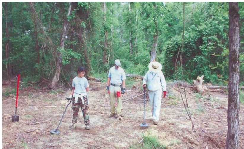
Instrument-assisted surveys help to identify the locations of spent munitions requiring removal from the Munitions Demolition Area (OD033).
